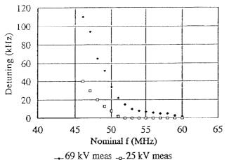
Figure 4. Cavity detuning due to ferrite nonlinearity.
