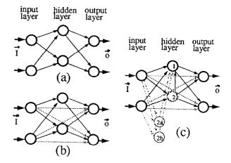
Fig. 2: Network connections: (a) Fully connected, (b) Shorcut connected and (c) Cascade network.
