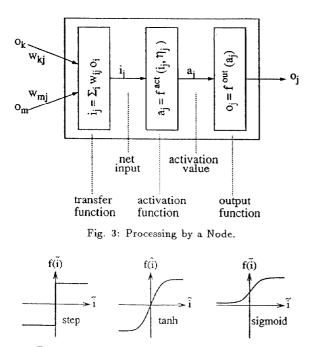
Fig. 4: Three frequently used activation functions
