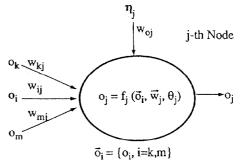
Fig. 1: Schematic representation of a Node
