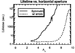
Figure 3. Lifetime versus horizontal aperture for LEP with and without errors.
