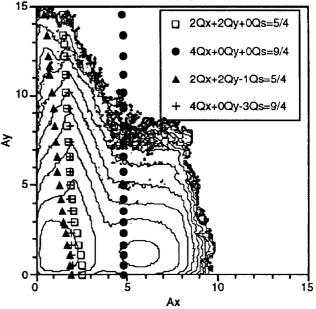
Figure 2. LEP beam-beam tail distribution with lattice including errors. The tunes in the legend refer to 1/4 of the total tunes.
