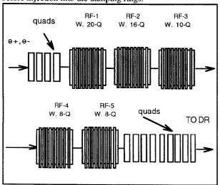
Figure 1. The layout of the SLC injector linac
