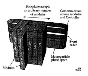
Fig. 3: The Software Back Plane and Model Elements
