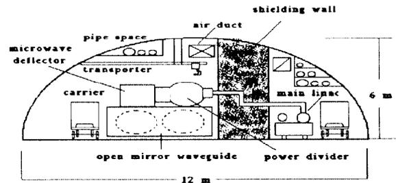
Figure 3: Placement of equipment in the accelerator tunnel
