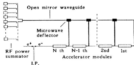
Figure 1: Linear collider scheme
