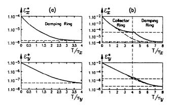
Fig. 3: Damping of the normalized transverse emittances of the electron (a) and positron (b) beams as a function of the circulating time, T, normalized to the damping time,  $\tau_{xy}$ .
