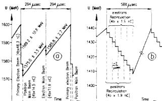
Fig. 2: Compensation of beam loading in the injector (a) and in the booster (b) linacs:
