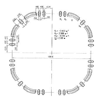
Figure 4. Lay-out of the DBA booster synchrotron (measures in mm).
