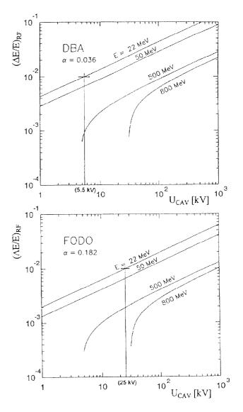
Figure 2. Energy acceptance of the booster synchrotron at 352.2 MHz for the DBA (upper part) and FODO structure (lower part).
