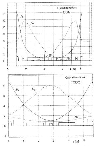
Figure 1. Lattice functions  $\beta_X$ ,  $\beta_y$ ,  $\eta_X$  and indication of the optical elements for the DBA (upper part) and FODO structure (lower part).
