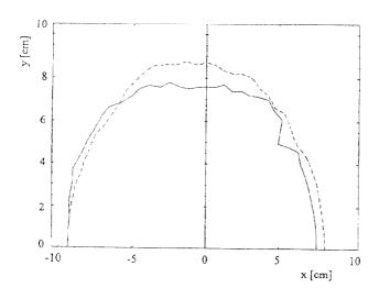
Figure 3. Dynamic aperture for DBA (full line) and FODO lattice (dashed line) at the nominal energy of 800 MeV.
