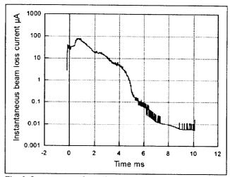
Fig. 3. Instantaneous beam loss current with time.
