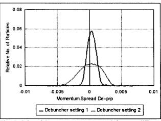
Fig. 7. Injected beam momentum spread for two different debuncher settings.
