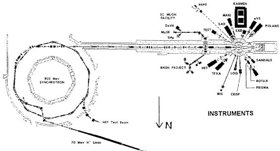
Fig. 1 ISIS accelerator and instrument lay-out.
