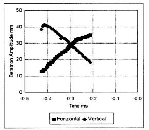
Fig. 5. Horizontal and Vertical betatron amplitudes during injection.
