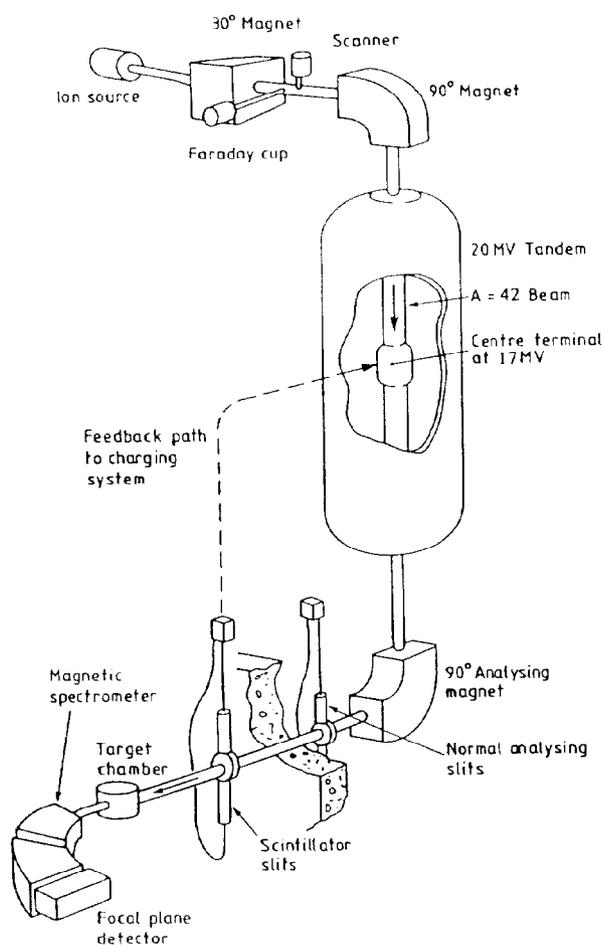
Figure 1: Use of NSF as an Accelerator Mass Spectrometer
