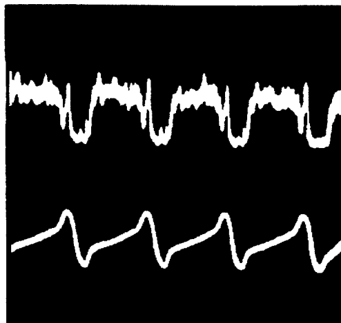
Fig. 5. The stretched beam (top) and the frequency program (bottom) in the phase displacement mode.
