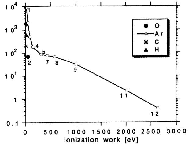
Figure 3: An argon plasma yield: we plot also some clearly identified impurities. The numbers indicate charge state.
