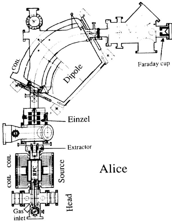
Figure 1: Section of Alice and its beamline.
