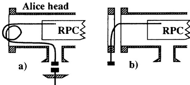
Figure 2: Detail of cooling water connection to the the removable plasma chamber: a) coiled tube with joint b) welded tube.
