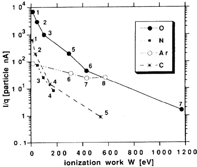
Figure 4: An oxygen plasma yield: note argon impurity.
