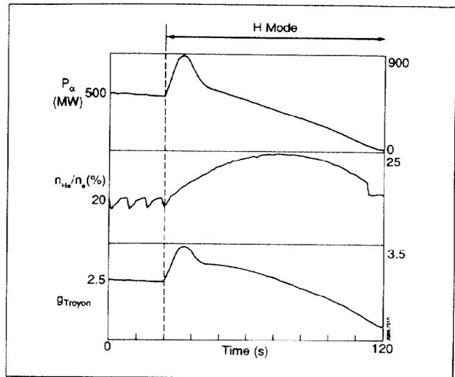
Fig.7: Long term deficiencies due to helium poisoning in the H-mode
