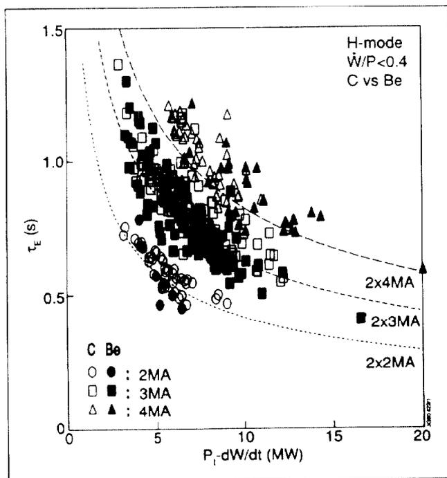
Fig. 2: Global energy confinement time ( $\tau_E$ ) during the H-mode as a function of net input power
