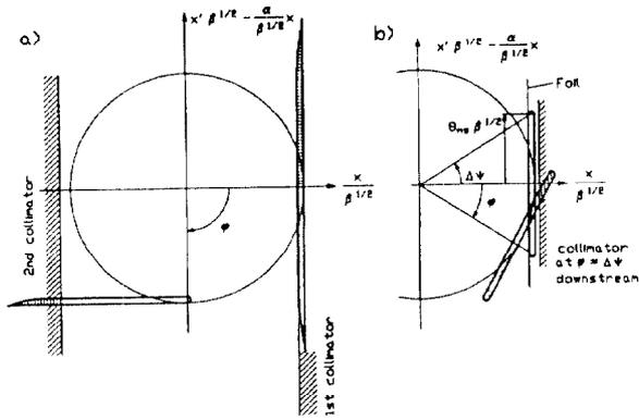
Figure 1: Multiple scattering out of a collimator (a) and by a scatter foil (b)
