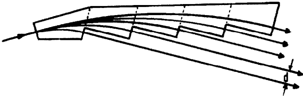
Figure 4: Scheme of a bending magnet. The dotted lines indicate the blocks.
