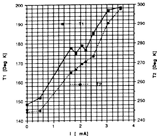
Fig. 2. Temperatures measured on the small diameter beam tube bellows at the cold/warm transition. T2 is at the conical transition, T1 in the middle of the bellows.
