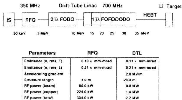
Fig. 1. Conceptual variable-energy 25-mA D<sup>+</sup> linac optimized for design current.
