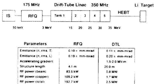
Fig. 2. Conceptual variable-energy 25 mA D<sup>+</sup> linac upgradeable to 125 mA.
