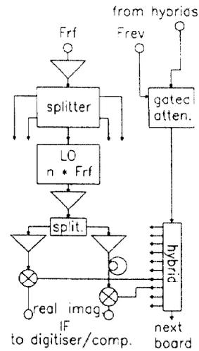
Fig. 2. RF Converter (one channel)
