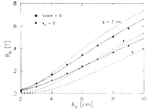
Fig.3 Field amplitude in a horizontal field undulator of the fig.2 type ( $g=20$  mm) for different block spacings, and in a conventional undulator geometry (various gaps);  $Br=1.1T$ ,  $h=period/2$ , 2D limit in both cases.
