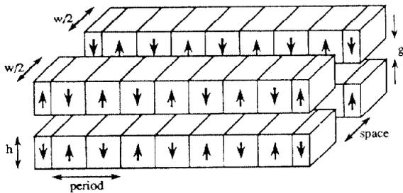
Fig.2 Planar permanent magnet array producing a periodic horizontal field distribution.
