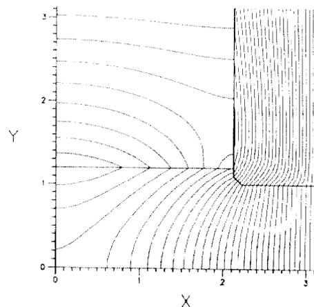
Fig.1 Field distribution in the multipole wiggler magnet.
