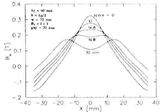
Fig.4 Field variation in the transverse direction for various block spacings
