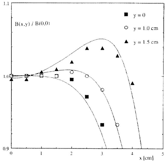
Fig. 3 - Calculated and measured (dots) ratio of the magnetic field to the centre value versus the distance  $x$  from the axis.
