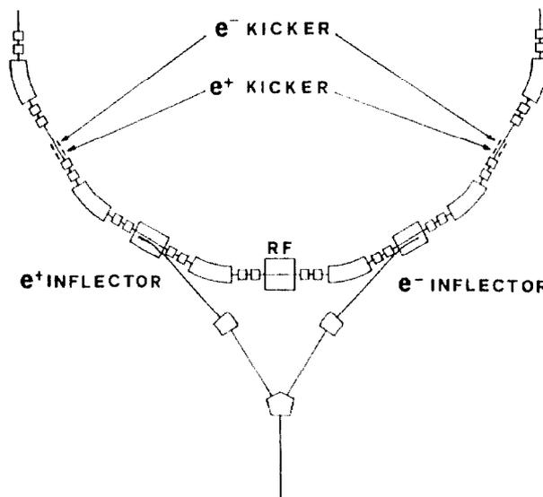
Fig. 1 - New electrons and positrons injection scheme with two pairs of kickers.
