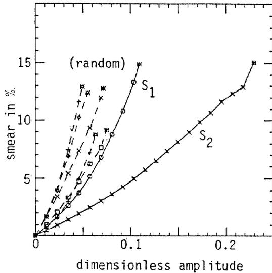
Fig. 1 Smear as a function of the dimensionless initial amplitude  $A_0$  ( $=A_x=A_y$ ) and dynamic aperture. Set No. 1 of Tables 1 and 2.
