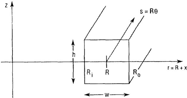
**Fig. 1: Toroidal beam tube geometry.**
