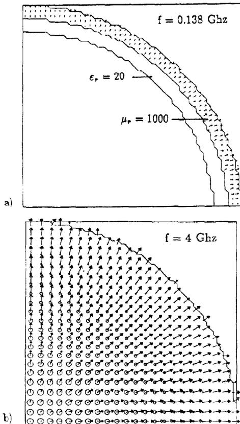
Figure 1:  $\vec{E}$ -Field of the lowest mode;  $k_z = 78 / m$
