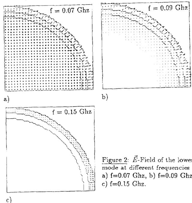
Figure 2:  $\vec{E}$ -Field of the lowest mode at different frequencies  $f$ ;
