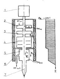
Fig. 1. Schematic lay-out of the magnicon: 1-electron gun, 2-cavity of the deflection system, 3 and 4-passive cavities of the deflection system, 5-cutput cavity, 6-solenoid, 7-collector.
