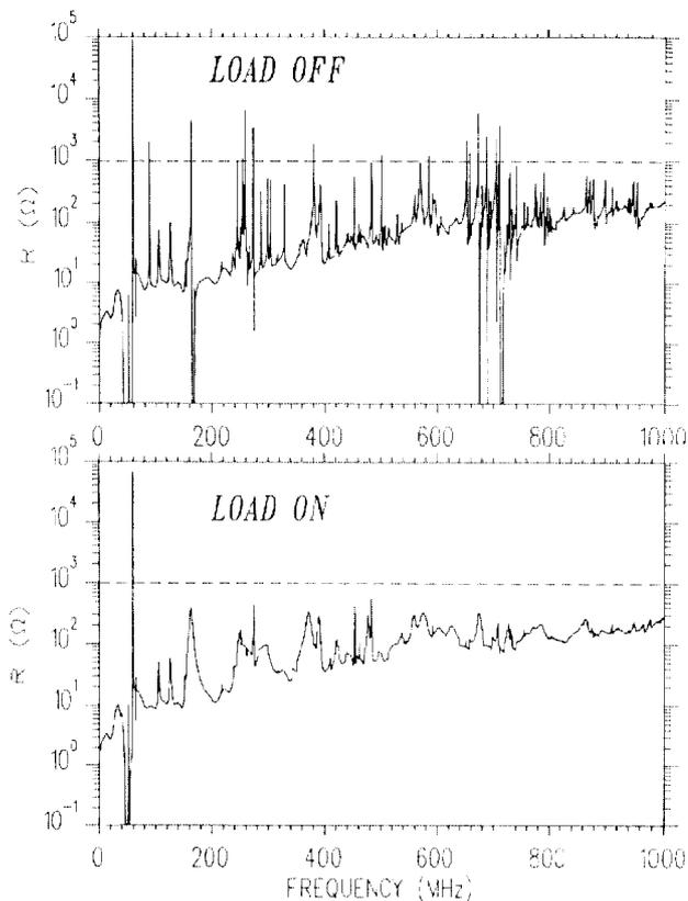
Figure 8: Shunt resistance of LAMPF cavity with damping resistors on and off
