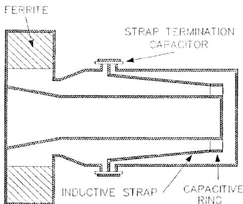
Figure 7: Cross section of LAMPF cavity showing strap termination capacitance
