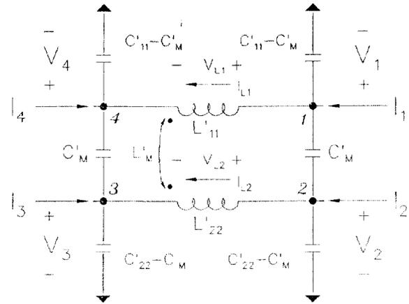
Figure 2: Lumped element representation of coupled transmission lines
