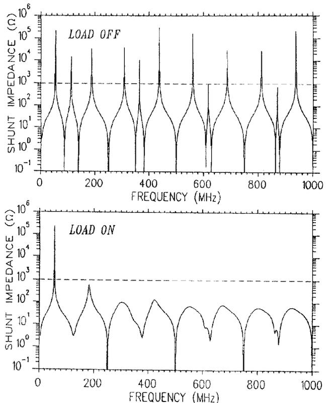
Figure 5: Shunt impedance of cavity with damping resistor off and on
