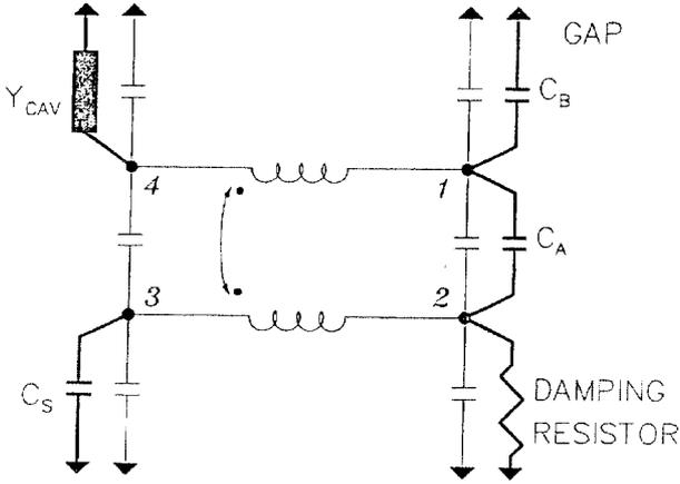
Figure 3: Lumped element representation of mode damper in cavity
