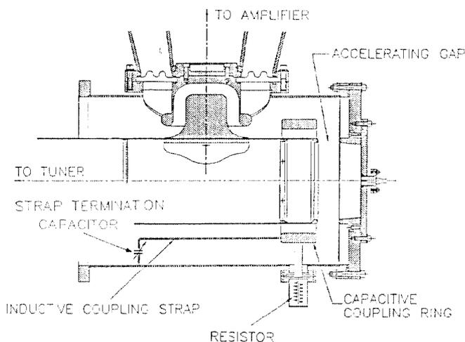
Figure 6: Coupled transmission line damper in LAMPF prototype booster cavity
