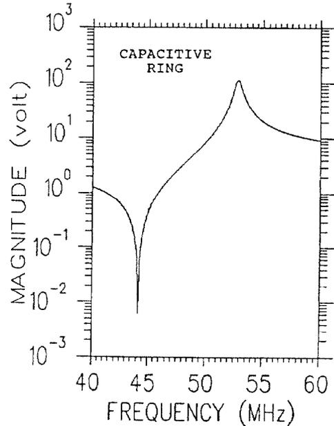
Figure 4: Voltage response on capacitive ring
