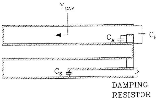
Figure 1: Coupled transmission line higher order mode damper
