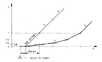
Fig. 2 - Slow start by stretching the first mini-vector from 256 to 1024 ms
