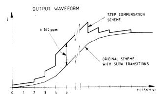
Fig. 4 - Compensation of the effects of the dipole vacuum chamber eddy currents by adding current offsets in the PC's of the quadrupole and sextupole circuits .
