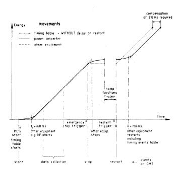
Fig. 1 - Timing events and equipment synchronization
