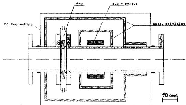
Figure 5: Mechanical layout of BCT
