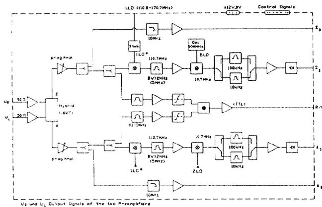
Figure 2: Blockdiagram of BPM-analogue electronics
