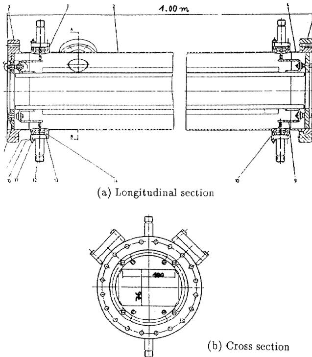
Figure 6: Mechanical design of Schottky pick-up
