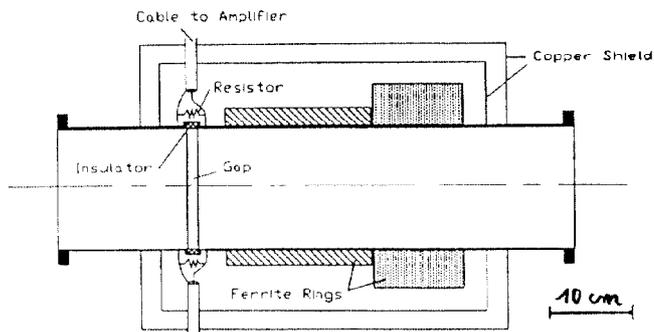
Figure 4: Mechanical layout of WCM
