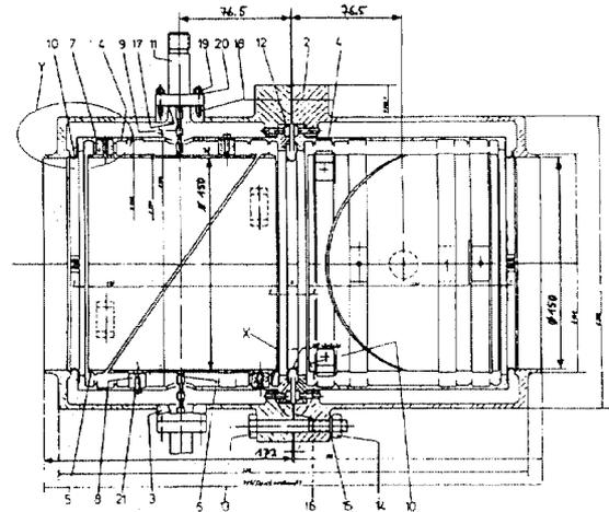
Figure 1: Mechanical design of the round BPM
