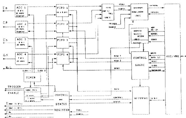
Figure 3: Blockdiagram of BPM-digital electronics
