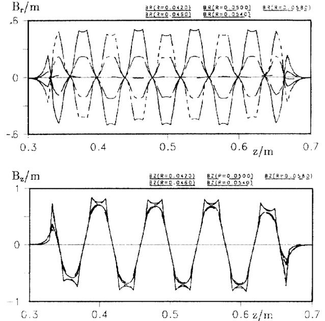
Figure 5: Magnetic field components  $B_z$  and  $B_r$  along  $z$ .
