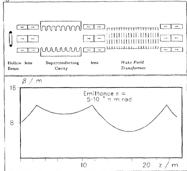
Figure 7: Section in the hollow beam driver linac. The collider consists of several normal cells like the one schematically given in the first picture. The corresponding radial  $\beta$ -function of the hollow beam on the cylinder with radius  $\rho$  is given below.
