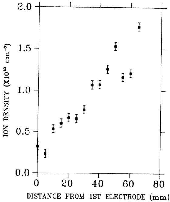
Fig. 2. Variation of the ion density on distance from the first electrode.
