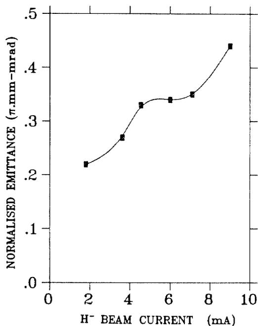
Fig. 7. Normalised emittance versus the extracted beam current up to 9mA.
