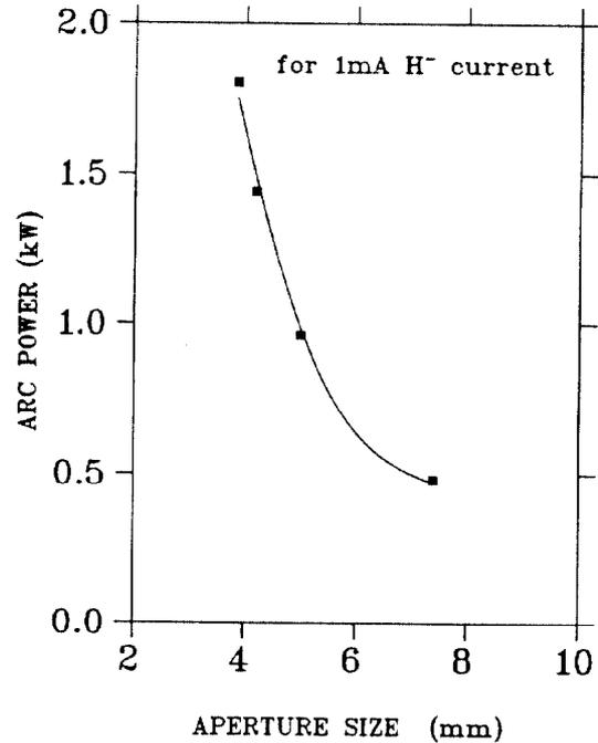
Fig. 5. Necessary arc power to obtain 1mA H<sup>-</sup> current for various apertures of the first electrode.
