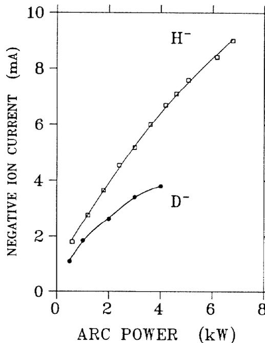
Fig. 8. Extracted H<sup>-</sup>/D<sup>-</sup> beam current versus arc power.
