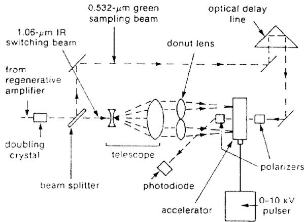
Figure 4: Schematic of electro-optic sampling setup.
