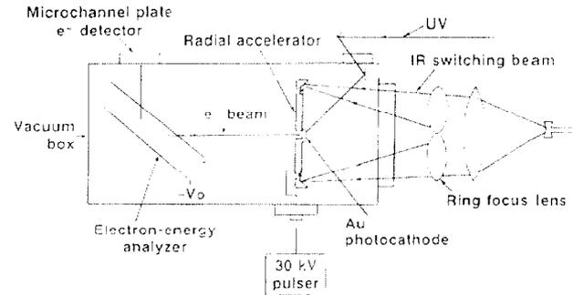
Figure 6: Schematic of electron acceleration setup.
