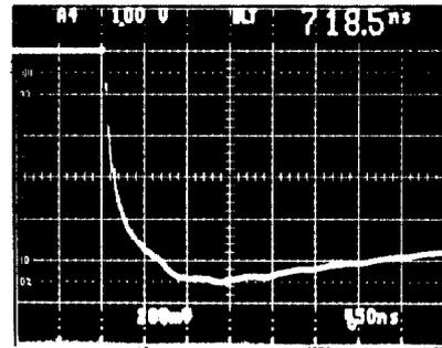
Figure 2: 1.5kV voltage pulse applied to the accelerator without the IR switching beam.
