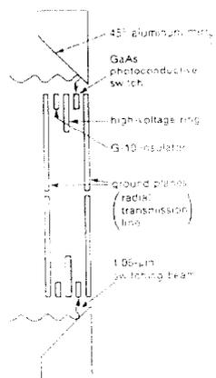
Figure 1: Schematic of the single stage radial accelerator.
