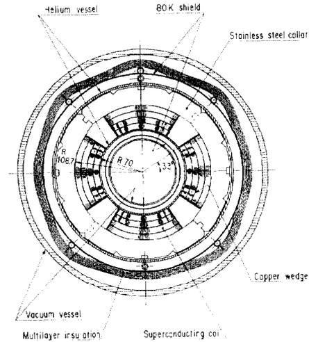
Fig. 5 Cross-section of the superconducting quadrupole magnet assembled in a horizontal cryostat.
