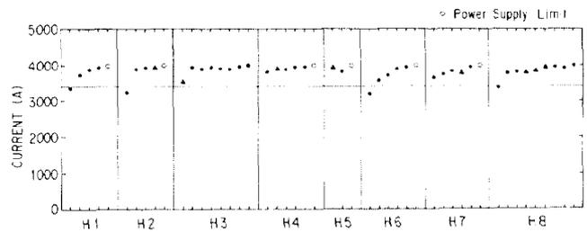
Fig. 6 Training behavior of the eight superconducting quadrupole magnets fabricated. Black circles and triangles indicate inner and outer coil quenches, respectively. White circles indicate the maximum currents of the power supply, and have been reached without quench.
