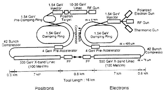
Fig. 8 Configuration of the JLC complex preliminarily designed.
