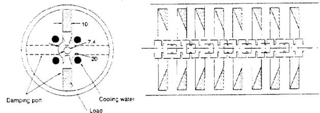
Fig. 9 Schematic drawing of an X-band structure with damped higher-order-mode Q's designed by use of a 3D computer code, MAFIA.
