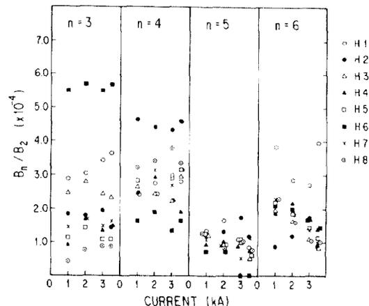
Fig. 7 Integrated harmonic contents measured for the eight superconducting quadrupole magnets fabricated.
