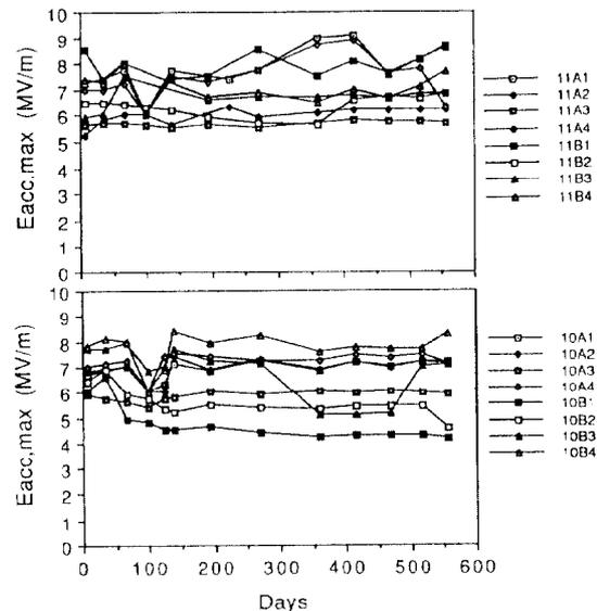
Fig. 3 Time variation of the maximum accelerating field for the 16 cavities installed in 1988 and operated for about 9000 hours.
