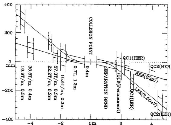
Fig. 11 A collision insertion of the asymmetric B-factory designed for a case of the head-on beam crossing.
