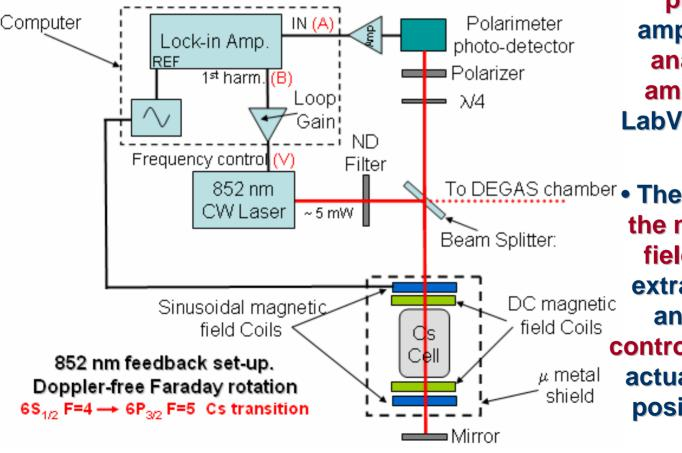
• The signal from the photodiode is then amplified, digitised and analysed by a lock-in amplifier developed in LabView and running on a PC computer.
