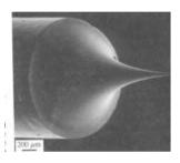
• The highest brightness source presently in operation is a field emission source for electron  $\delta \approx 10^{-5}$  microscope applications, where the tip is a carbon nanowire. For this source:
