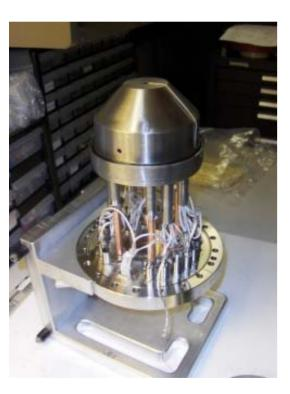
Contacts between different metals in the parts inside the magnetic shield have been carefully avoided in order to not generate local voltages and/or currents and thus undesired stray fields.
