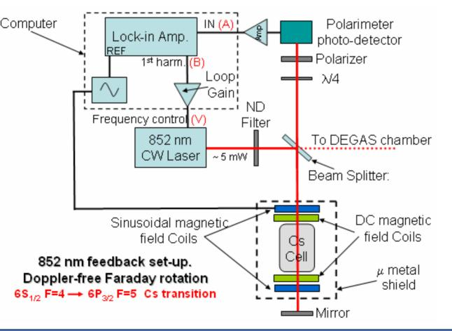
• A sinusoidal signal is applied to one of the coil sets to generate a magnetic field of few tens of mG and ~ 100 Hz frequency.
