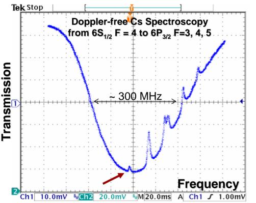
• The interaction between the electron and the magnetic field of the nucleus generates a hyperfine structure on the Cs levels that shows as a set of local peaks in the transmission curve (some of the peaks are also due to the excitation of atoms with different group velocity).
