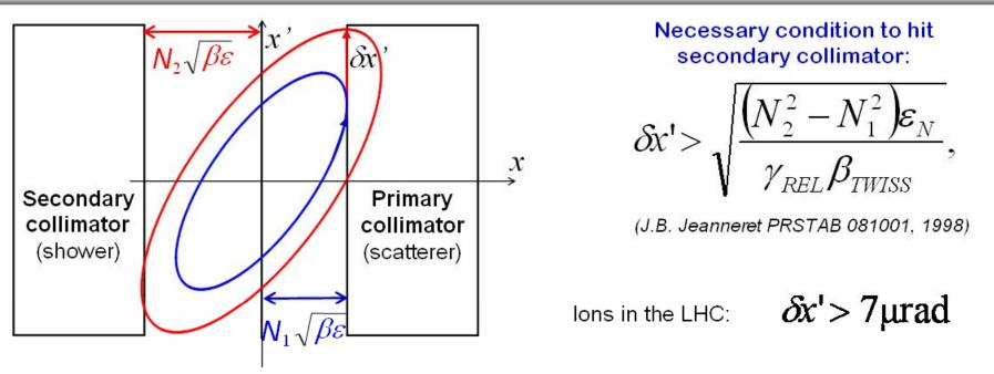
RMS MCS angle of 2.76 A TeV Pb<sup>82+</sup> ions on graphite:  $\sim 4.7 \mu \text{ rad/m}^{1/2}$
