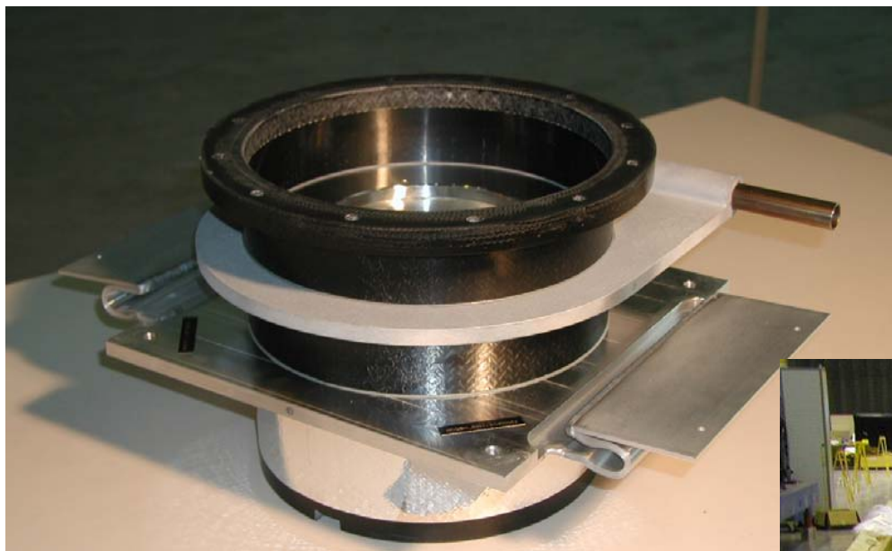
Low heat leak GFRE support post
