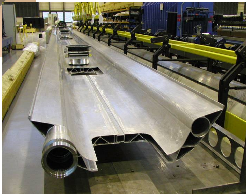
Aluminium extrusion for thermal shield
