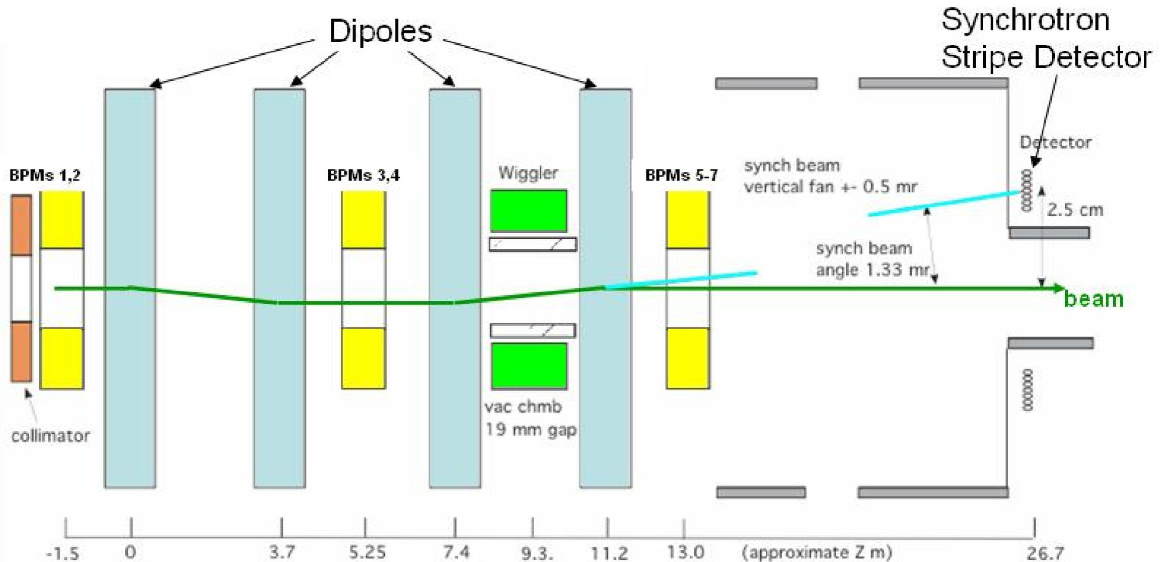
**Figure 3-1.** Plan view of 4-dipole chicane with vertical wiggler magnet for energy spectrometer studies. Two additional BPM doublets are 10 meters and 50 meters upstream of BPMs 1, 2 respectively. Not shown is an interferometer system measuring horizontal offsets and stability of BPMs 1-4.
