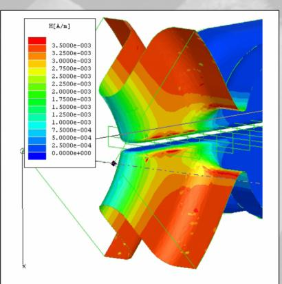
Figure 2.10: Magnetic field distribution on the cell walls of an HDS CLIC prototype structure. The magnetic field distribution in the figure  $(H \ [A/m])$  is given for 1 MV/m accelerating gradient. For fixed geometry the magnetic field is proportional to gradient, so for 100 MV/m H need to be multiplied by 100. ©Alexej Grudiev, CERN
