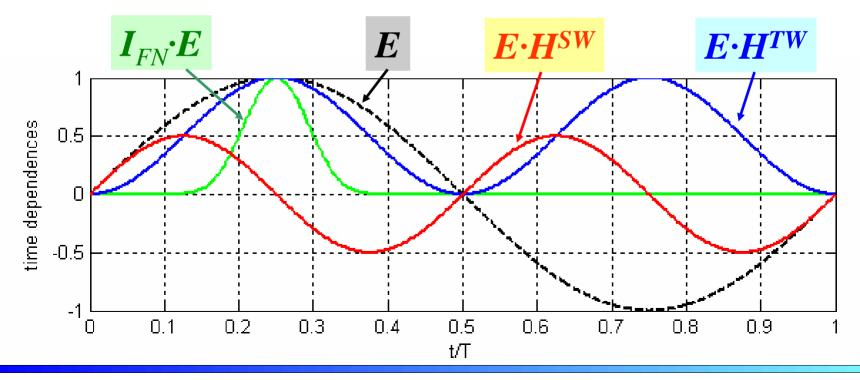
What matters for the breakdown is the amount of rf power coupled to the field emission power flow.
