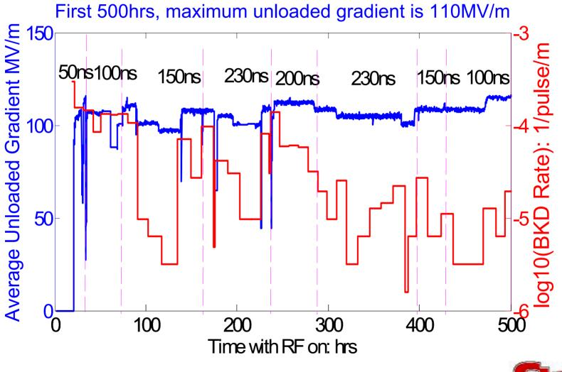
The BKD Rate is normalized to the structure length(29cm)
