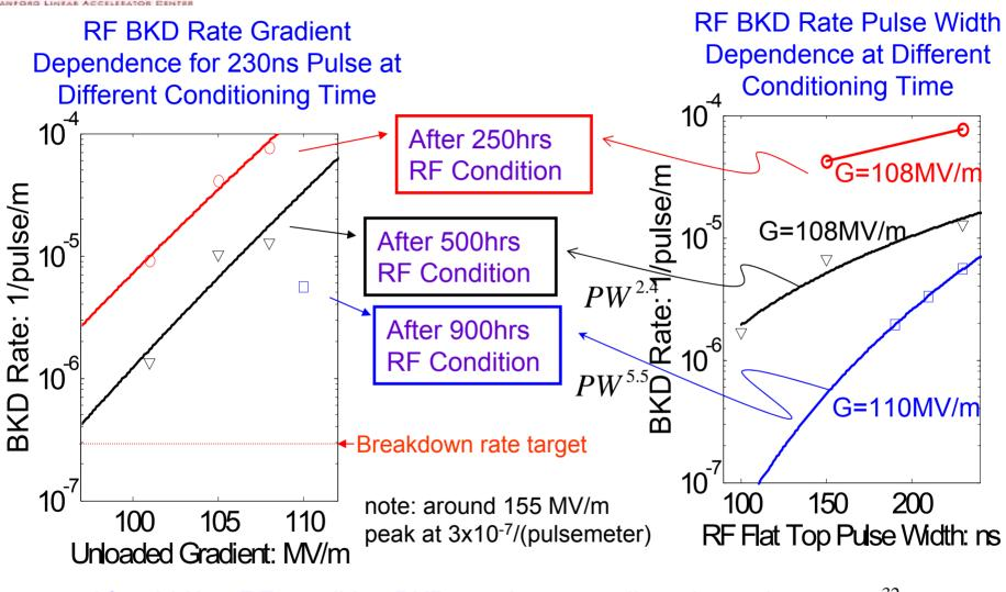
After 900hrs RF condition BKD rate has a gradient dependence ~  $G^{32}$ and pulse width dependence ~  $PW^{5.5}$
