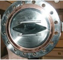
In-situ bakeout to activate the NEG at 180°C, kapton foils (thickness <0.4mm) with printed circuits used for the bakeout.
