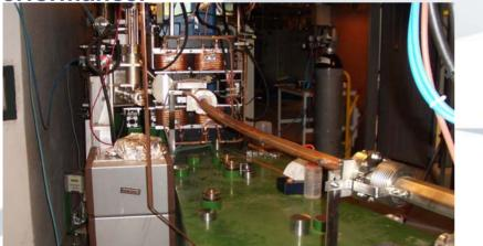
COURTESY OF E. Wallén, Test of a NEG Coated Copper Dipole Vacuum Chamber, these proceedings.
