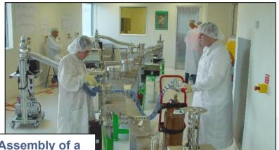
Assembly of a complete sector (incl. the gate valves ), pump and leak test.
