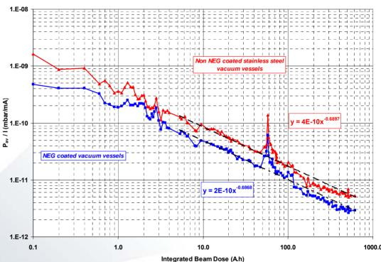
Average pressure of Cell C07 normalised to current Vs. the beam dose
