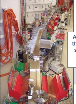
Assembly of the complete sector over the open magnets.
