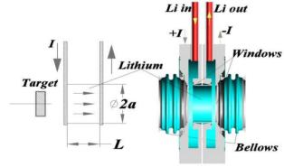
Figure 1: Lithium lens concept, left. At the right the transverse cut or suggested lens design is represented.
