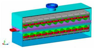
Figure 3: 11-pole wiggler cold mass. Two side walls removed. Room temperature vacuum chamber and 70°K shield are seen also.
