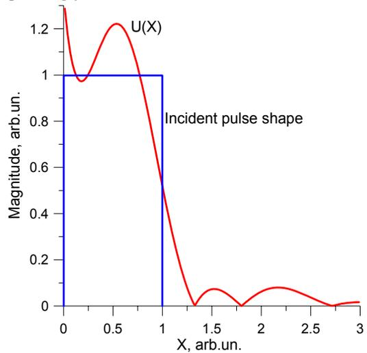
Figure 6: Leakage of power from optimized three-mode cavity (red curve) and the desirable pulse shape (blue curve).
