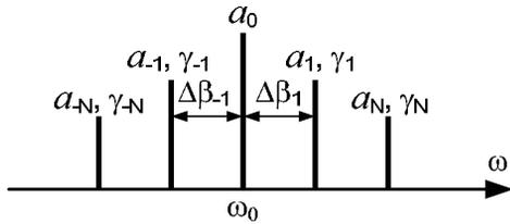
Figure 4: Necessary spectrum of leaky eigen waves.
