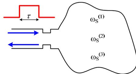
Figure 3: Feeding of multi-mode cavity.
