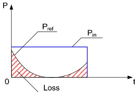
Figure 2: Input and reflected pulse shapes in regime of power storage in single-mode cavity.
