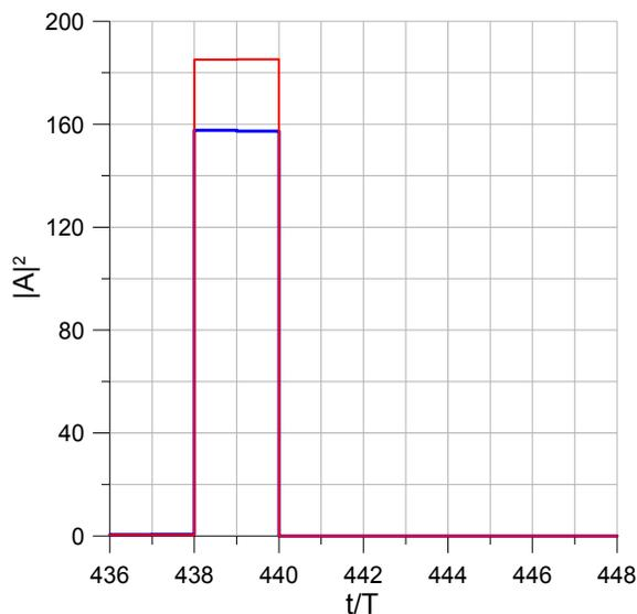
Figure 10: Output pulses of single-mode and two-mode SLED-II compressors.
