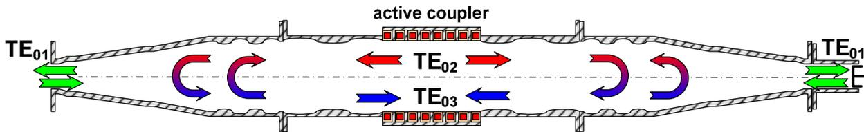
Figure 9: Double-mode TE01-TE02-TE03 pulse compressor.
