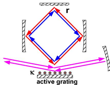
Figure 8: Double-mode four-mirror pulse compressor.
