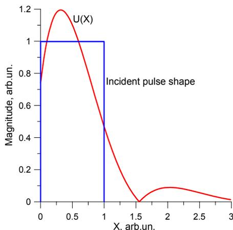
Figure 5: Leakage of power from optimized double-mode cavity (red curve) and the desirable pulse shape (blue curve).
