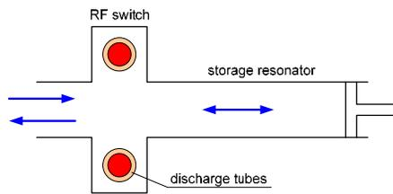
Figure 1: Active pulse compressor.
