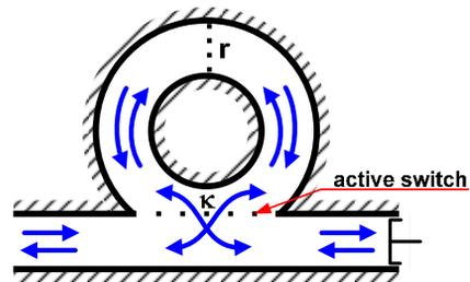
Figure 7: Model of traveling wave cavity.
