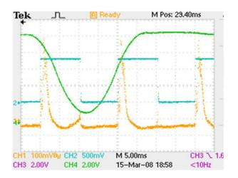
Figure 2. First operation of the MICE target with beam. The signals shown are the target trajectory (arb. units, green), circulating intensity in ISIS (blue) and the ISIS beamloss sum signal (yellow). The beamloss signal shows a rise at  $\sim$ 6-10ms as the MICE target is inserted. No interference is seen with subsequent ISIS pulses.
