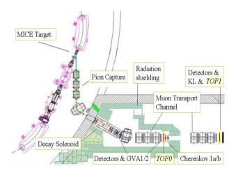
Figure 1. Layout of the MICE muon beamline
