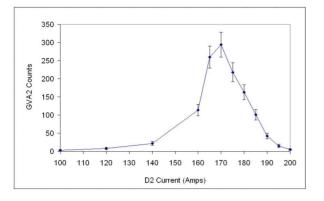
Figure 3. Recorded hits in detector GVA2 against current in second dipole.
