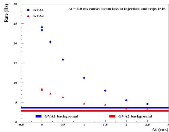
Figure 5: Rates of proton counts in scintillation counters GVA1 (circles) and GVA2 (triangles) placed in the MICE beam-line, plotted as a function of target delay,  $\Delta t$ , for a constant dip depth after the optimum insertion time. The one-standard-deviation background rate bands are shown for GVA1 (upper band), and GVA2 (lower band).
