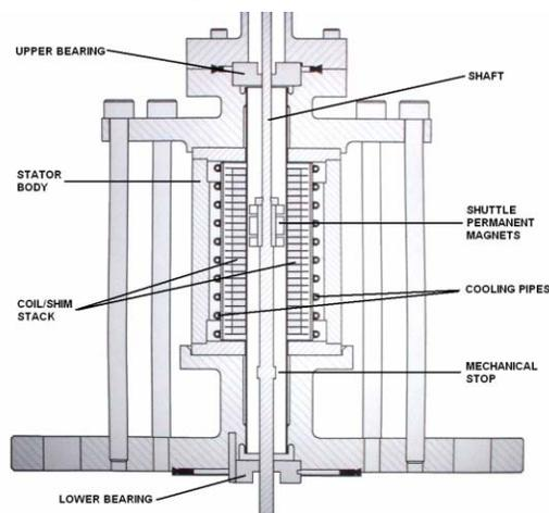
Figure 1: The stator mounted in its supporting flanges. The stator body with its end caps measures 90mm. (Note that the full length of the target shaft [560mm] and the optical readout block are not illustrated.)
