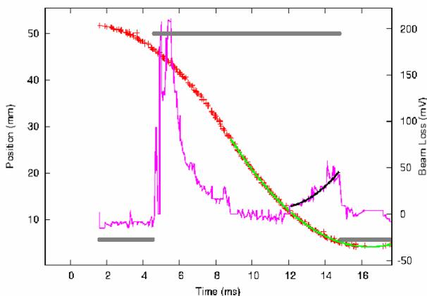
Figure 4; Illustration of the target trajectory (curved line - mm) and its relationship to beamloss (noisy line - mV). The large spikes on the LHS of the beamloss are due to ISIS injection losses. Losses caused by the target can be seen as the rise in the beamloss signal on the RHS of this signal (fitted). The top hat signal (solid line) shows when the beam was on in ISIS (10ms).
