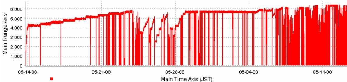
Figure 8: Power history during the measurement of BDR at 300 ns. The vertical axis corresponds to RF power.
