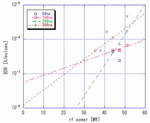
Figure 9: Breakdown rate as a function of a pulse width of #SUS003.
