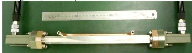
Figure 1: Narrow waveguide of stainless-steel (#SUS003).
