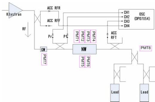
Figure 3: Measurement system of RF pulses.
