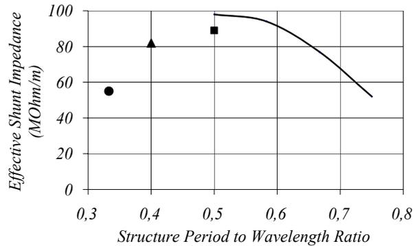
Figure 3: Effective shunt impedance. Curve - STW structure, square - SW structure, triangle- BTW structure, circle - disk-loaded waveguide.
