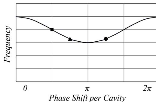
Figure 1: Dispersion diagram. Square – SW structure, triangle – BTW structure, circle – STW structure.
