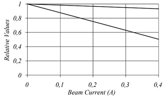
Figure 5: Field intensity in bunching section (upper line) and output electron energy (lower line) in relation to beam current.
