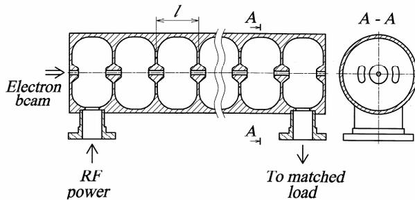
Figure 2: STW structure (front and side views).
