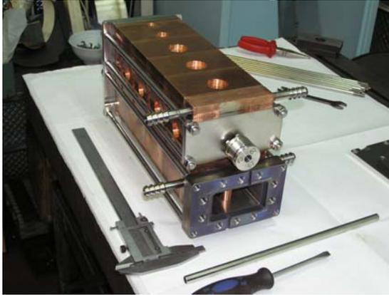
Figure 3: The parallel coupled accelerating structure.
