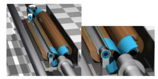
Figure 3: Rotatable Jaw Collimator FLUKA Layout.
