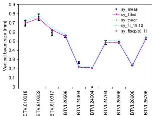
Figure 7: Fitted vertical beam sizes, from screen BTV images, compared with their theoretical values..
