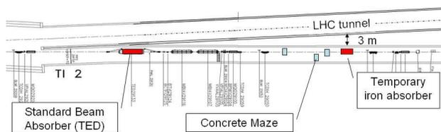
Figure 3: Temporary iron absorber and wall thickness between the two tunnels.
