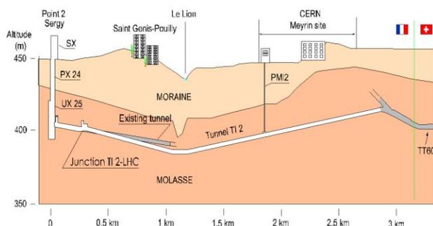
Figure 2: Vertical projection of the TI 2 transfer line.
