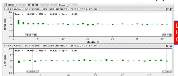
Figure 5: Horizontal and vertical trajectories after correction.
