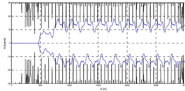
Figure 8: Measured (blue) and theoretical horizontal aperture throughout the TI 2 transfer line.
