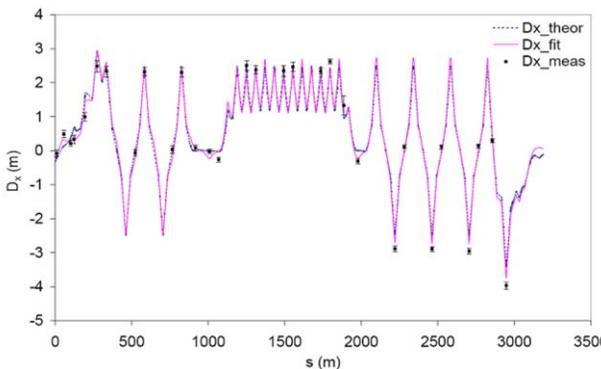
Figure 6: Comparison between measured and theoretical horizontal dispersion.
