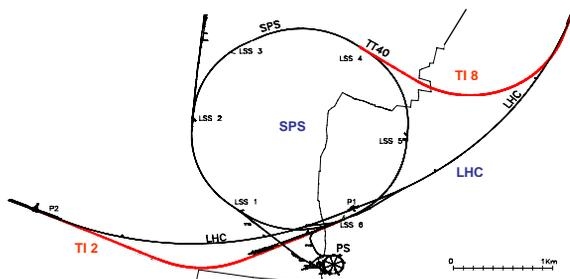
Figure 1: Layout of the LHC Transfer lines TI 2 and TI 8.
