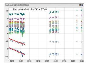
Figure 4: History of MKD "End" point in % relative amplitude, for 2007 running.
