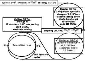
Fig. 1. Schematics of the NICA accelerator complex with parameters for U-U collisions.
