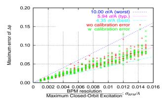
Figure 2: BPM resolution dependency of the betatron phase reconstruction error. The red and green points correspond to the simulation results with and without  $\pm 4\%$  BPM calibration error.
