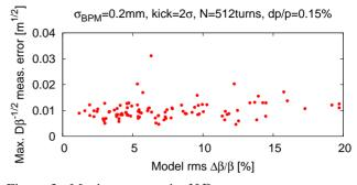
Figure 3: Maximum error in ND measurement vs. rms  $\beta$ -beating (simulation) for a 100 of LHC machines with errors.
