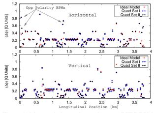
Figure 4: Measured phase advance between RHIC BPMs after trimming  $1^{st}$  set of three quadrupoles (blue) and the  $2^{nd}$  set (black) compared to the ideal model (red). Vertical error bars are statistical deviation between three consequetive data sets with the same condition
