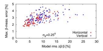
Figure 1: Maximum error in arc  $\beta$  measurement vs. r.m.s. model beta-beating. Phase error is assumed  $\sigma_{\phi} = 0.25^{\circ}$ .
